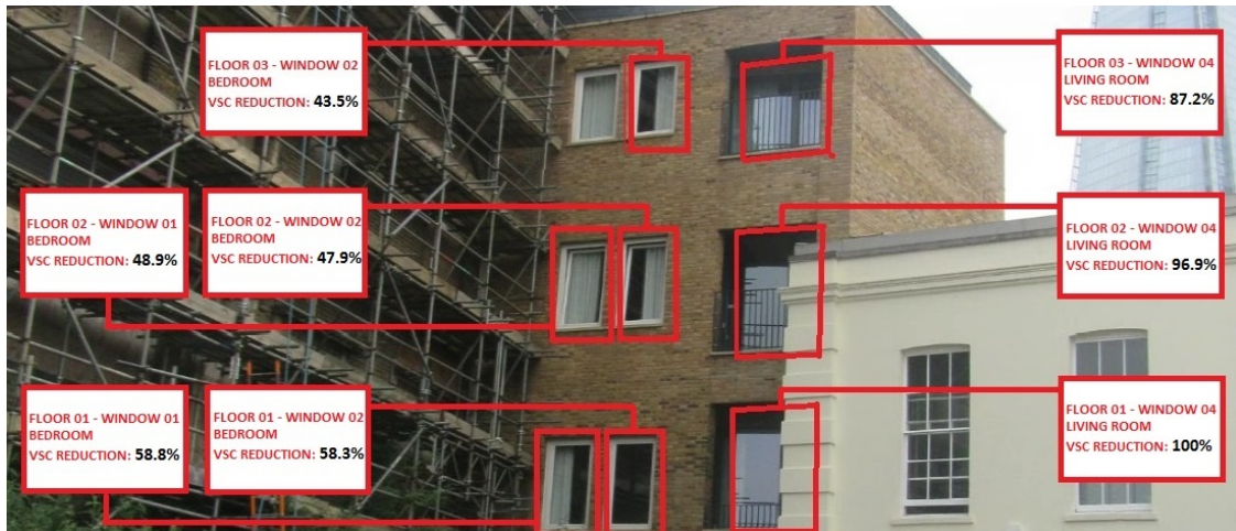
Figure 24: Window map of the west elevation of 11 Southwark Street highlighting those apertures that would experience a substantial adverse reduction in VSC
