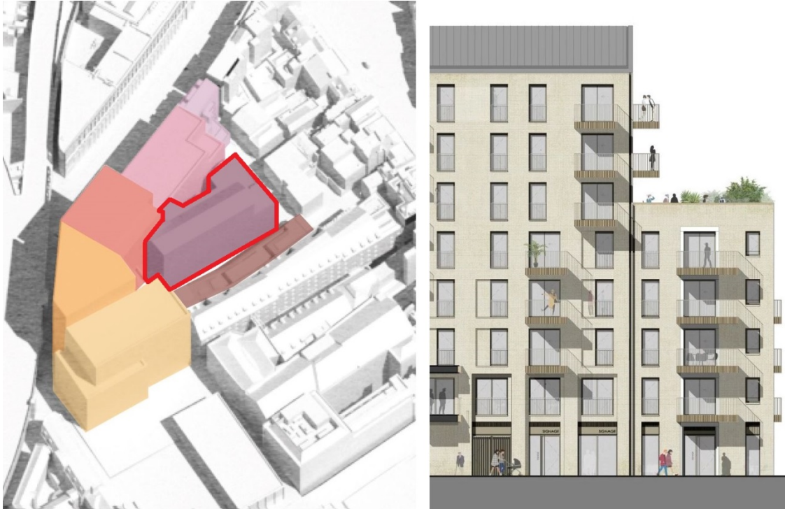
Figure 16 (left): Site diagram showing the proposed Residential East Building edged in red Figure 17 (right): Part of the south elevation of the Residential East Building, showing the relationship between the five-storey and eight-storey elements
