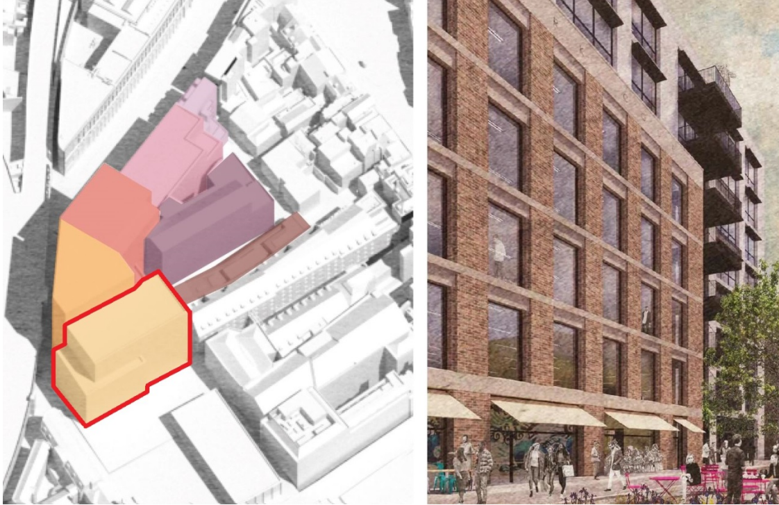
Figure 14 (left): Site diagram showing the proposed Woods Yard Building edged in red Figure 15 (right): Visualisation from Redcross Way looking eastward across the proposed Woods Yard public square. In the foreground is the red brick lower mass of the Woods Yard Building, with the white brick taller mass visible behind.
